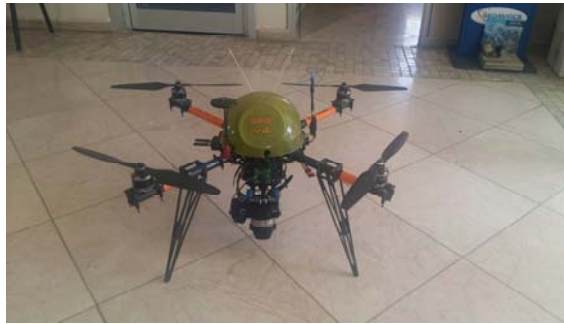
Fig. 1 GEO_2 UAV and environmental equipment
