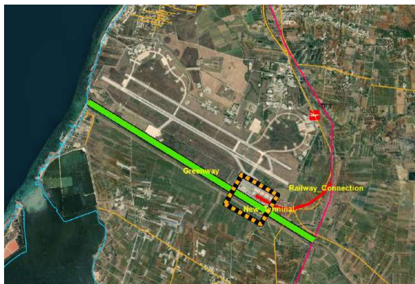
Fig. 9 Idea for a design planning of the node. 1) Connection to the railway; 2) Adequate, new terminal; 3) Green road to protect the existent canal to the sea (Font: Authors)
