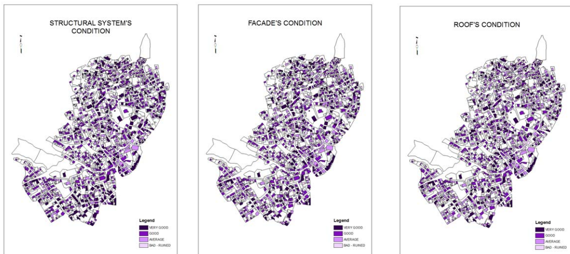
Fig. 4 a) Structural system's condition; b) Façade's condition; c) Roof's condition
