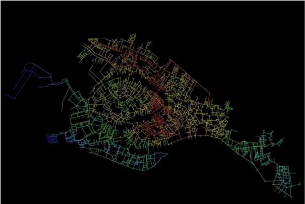
Fig. 7 The distribution of global integration value in the lines of the axial map of Venice (with 'traghetto')
