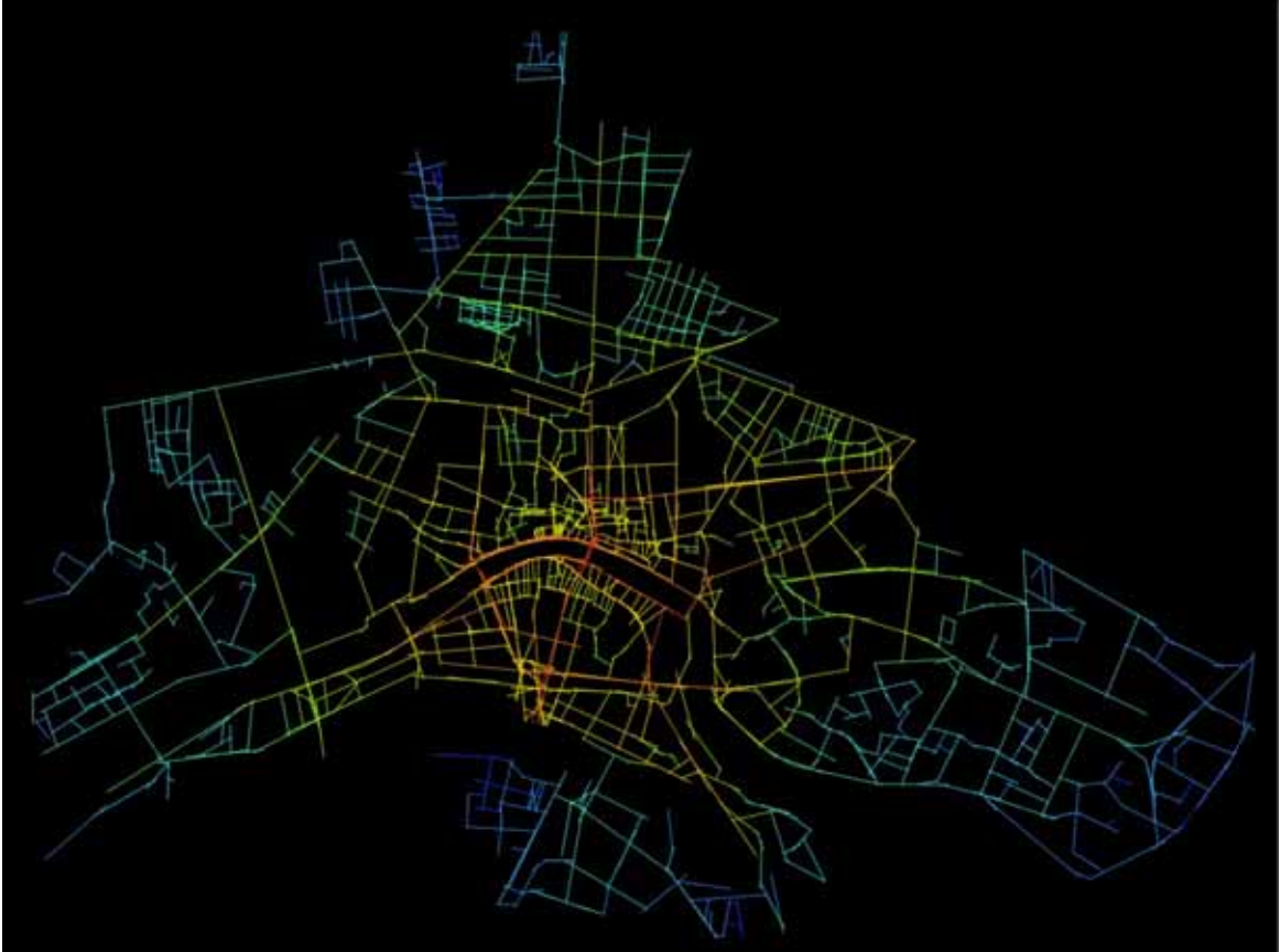
Fig. 5 The distribution of global integration value in the lines of the axial map of Pisa
