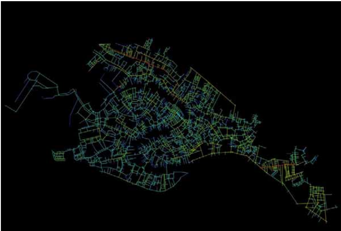
Fig. 10 The distribution of local (radius3) integration value in the lines of the axial map of Venice (with 'traghetti')
