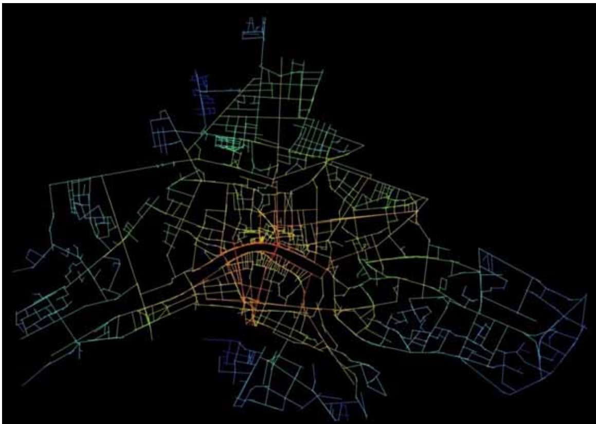
Fig. 12 The distribution of global integration value in the transformed axial map of Pisa
